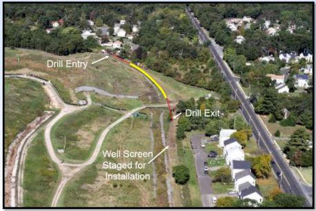
Horizontal Hydraulic Control Well for Landfill Leachate Containment
