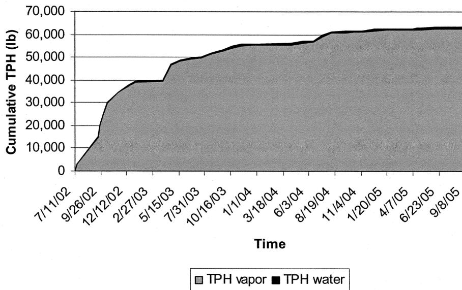
Figure 4. Total hydrocarbon removal.
