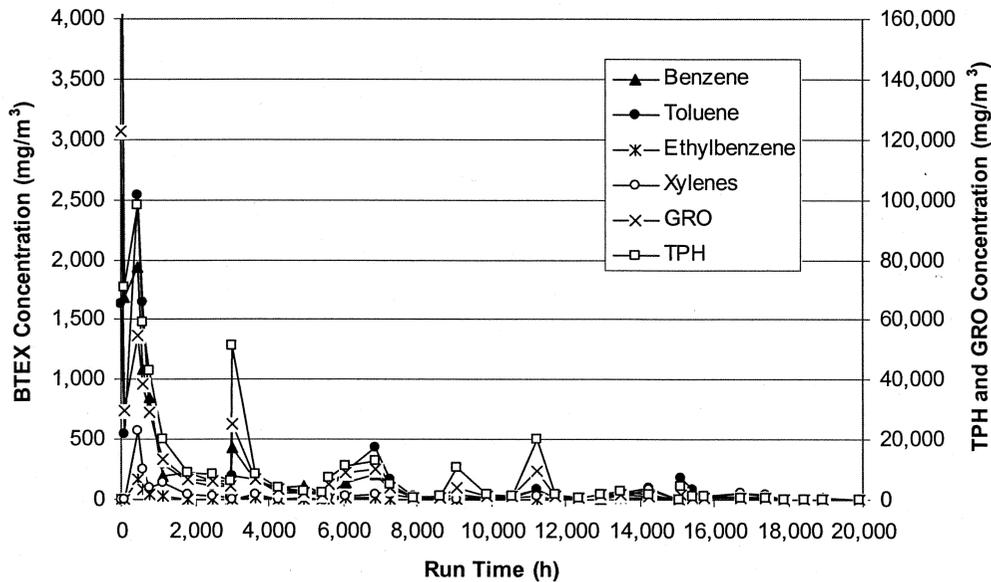
Figure 2. Hydrocarbon concentration trends in offgas since system start-up (initial data points exceed concentrations represented in figure).
