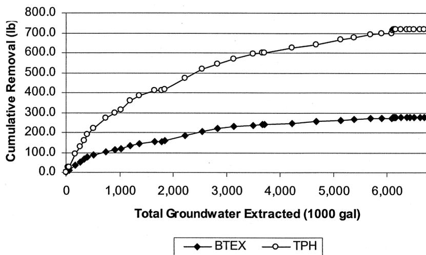
Figure 3. Cumulative TPH and BTEX removal – liquid phase.
