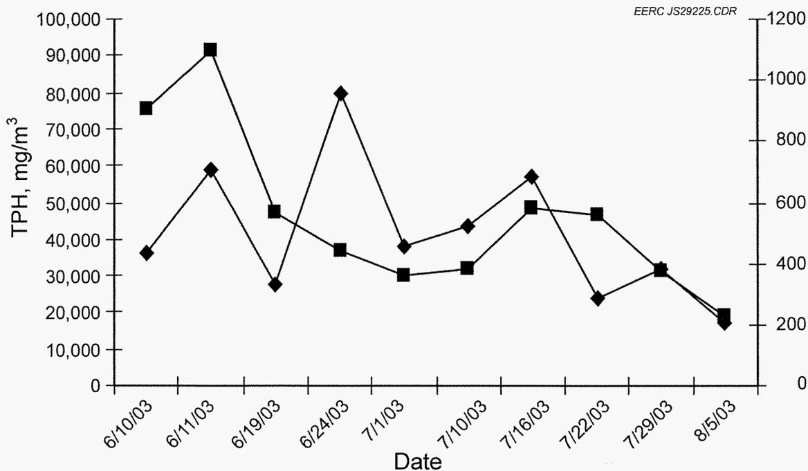
Figure 4. Hydrocarbon concentration trends in offgas – source area 2003.
