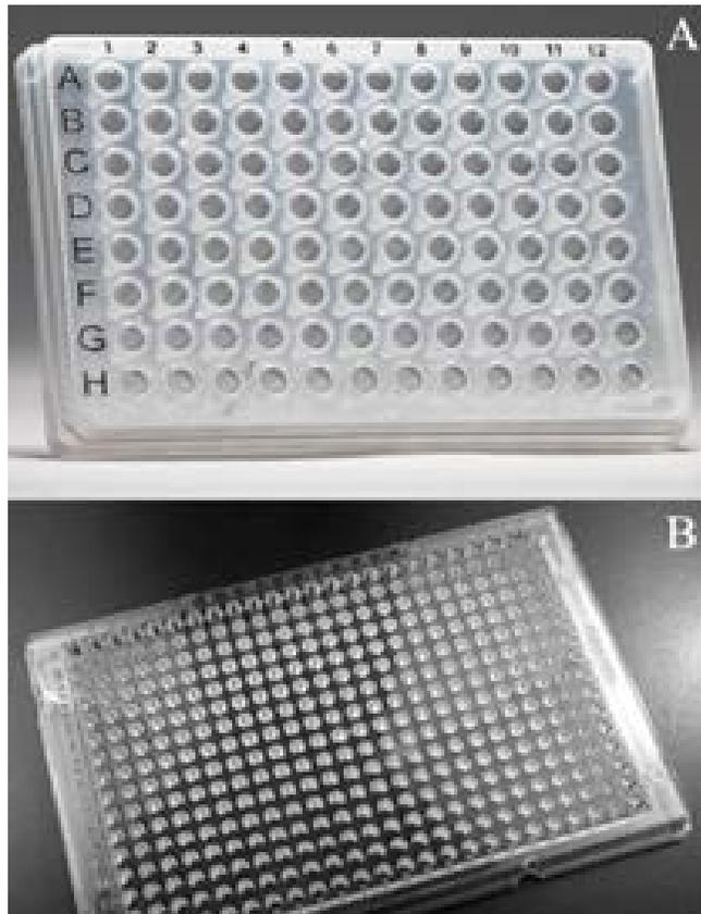
**Figure 4.** A) 96-well and B) 384-well qPCR plates
