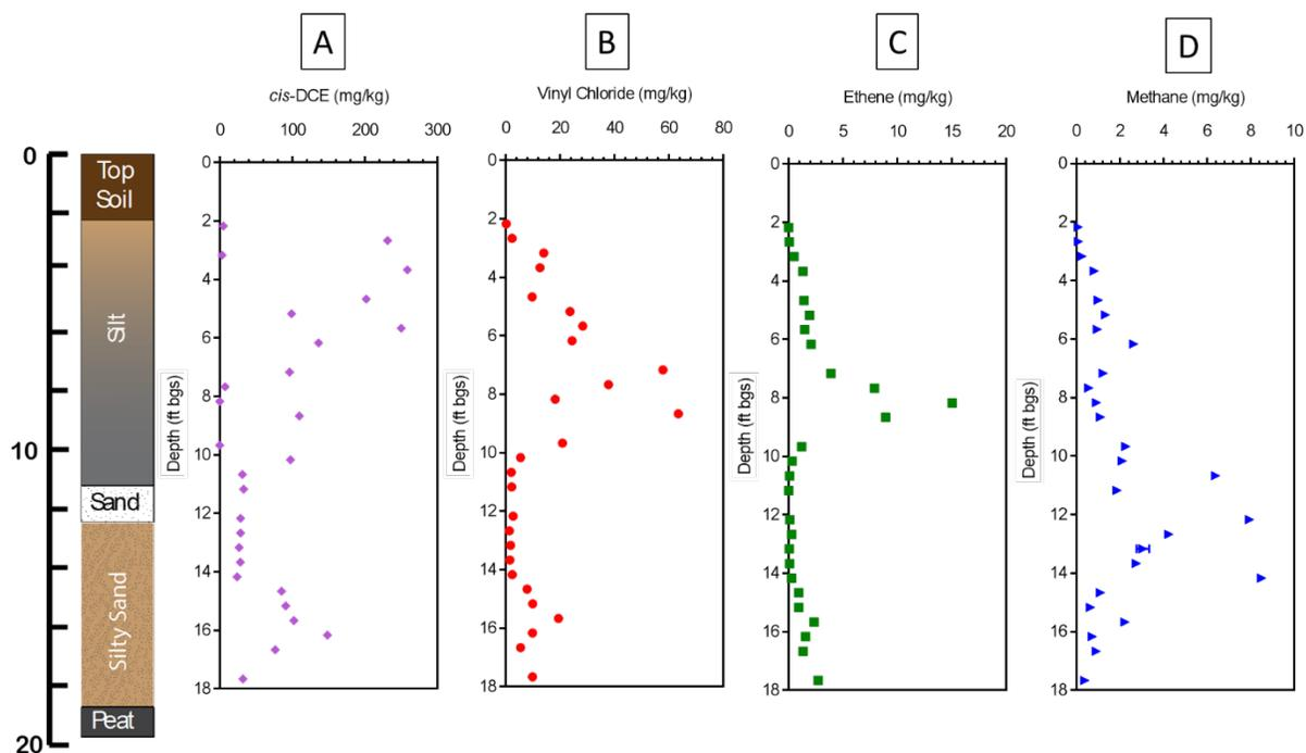
**Figure 8.** Spatial resolution of A) cDCE, B) VC, C) ethene, and D) methane in an aquifer sediment core, frozen in place with liquid nitrogen, obtained from Parris Island Site 45. The graphic on the left shows the soil characteristics of the upper (silt) and lower (silty sand) surficial aquifers.
