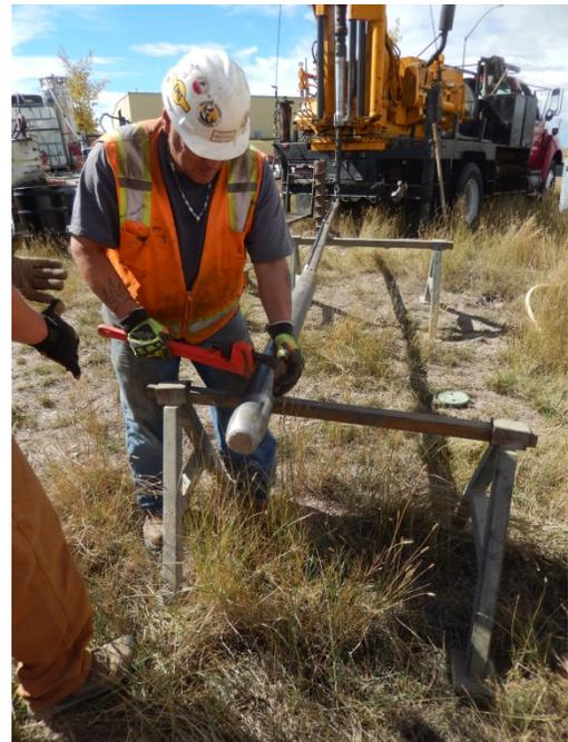
v. Remove the core sleeve from the core barrel
