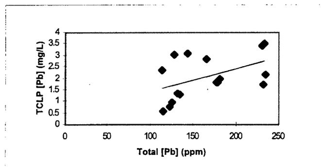
**Figure 30. TCLP vs. Total (Pb) Hydrochloric Acid Demonstration;**
