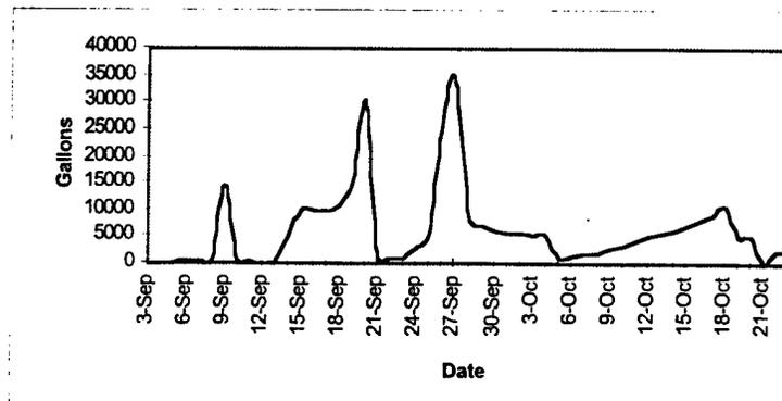
Figure 5. Estimated Runoff Pond Volume Acetic Acid Demonstration
