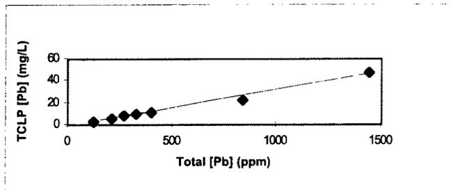
**Figure 29. TCLP vs. Total (Pb) Acetic Acid Demonstration;**
