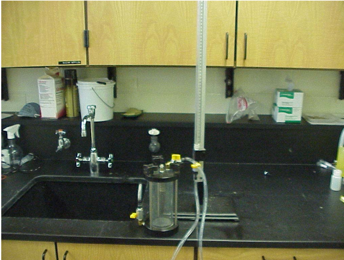
Figure 4-3. Humboldt HM-3891 permeameter.
