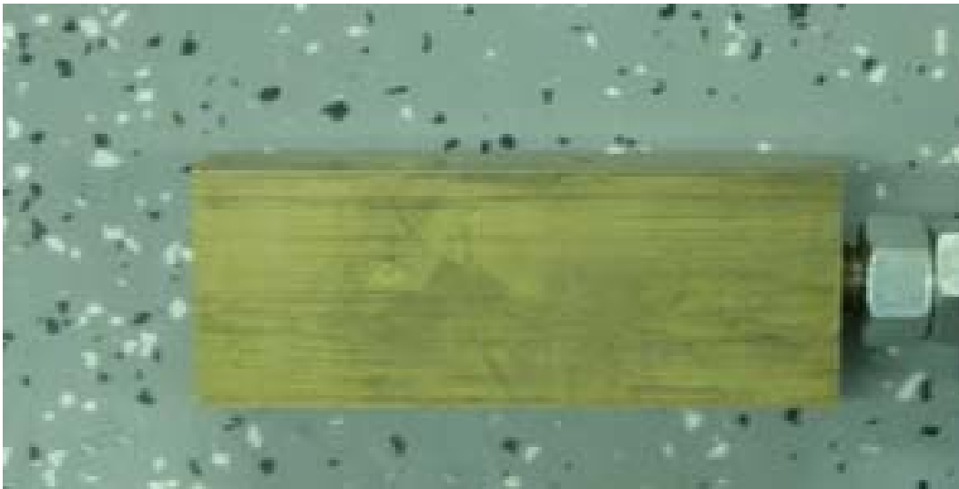
Figure 4-5. Close up view of compaction hammer head.
