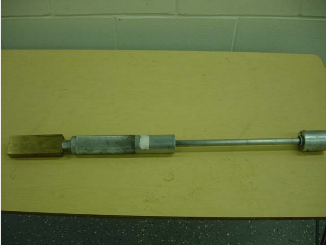
Figure 4-4. Modified compaction hammer used for compaction of bulk density and UCS samples.
