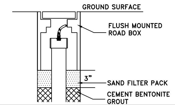
TYPICAL BELOW GRADE SVE/AI WELL COMPLETION DETAIL
