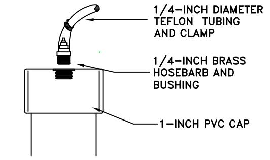
TYPICAL BELOW GRADE VAPOR PROBE DETAIL
