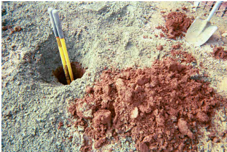
Figure 5-3. Installation of Thermocouples
