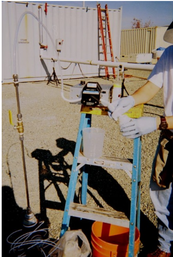
Figure 7-1. Groundwater Being Collected from BAT-06 Monitoring Well
