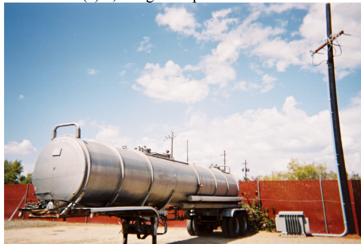
(b) 6,500-gal mobile Wastewater Disposal Tank
