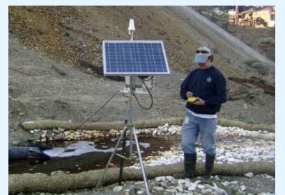
Water monitoring at the New Idria Mercury Mine Superfund site in California involves use of time-interval sampling devices powered by solar energy. Collected sampling data are transmitted via satellite to a website accessible by project staff. This approach supplies a renewable source of onsite energy and reduces the frequency of staff visits to this remote site. Ongoing investigation of this site led to removal actions in 2011 and 2015.
