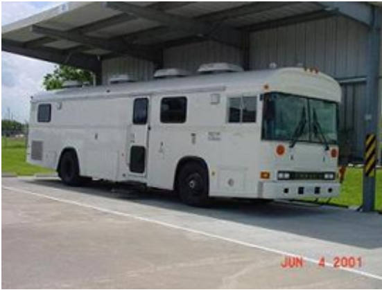
The trace atmospheric gas analyzer (TAGA) van is a self-contained mobile laboratory with specialized sampling equipment for measuring indoor air. TAGA equipment can provide analytical results for concentrations reaching the low parts per billion.
