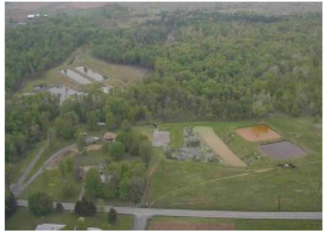
**Two Passive Treatment Systems:** Water is intercepted and diverted to the De Sale Phases 1 and 2 treatment systems where it is conveyed via gravity flow through multiple passive treatment steps.
