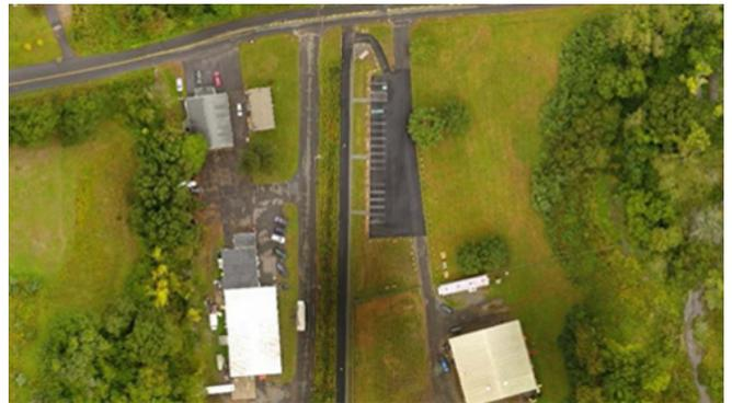
**Nature-Based Stormwater Controls:** The workplan for cap construction integrated nature-based techniques to control stormwater during long-term remedy operation and maintenance. Vegetation clearing was limited, impervious surfaces were converted to vegetated surfaces where feasible, vegetated swales were installed, and a vegetated filter strip was established near the onsite asphalt-surfaced parking lot.
