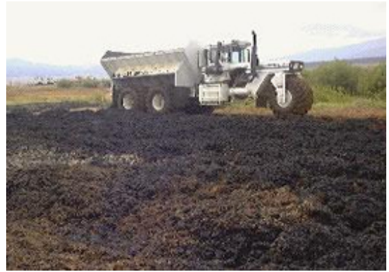
Biosolids from the Denver metropolitan area were applied at a rate of approximately 100 dry tons/acre and mixed with similar amounts of lime. Amendments were tilled into the soil to a depth of 12 inches.
