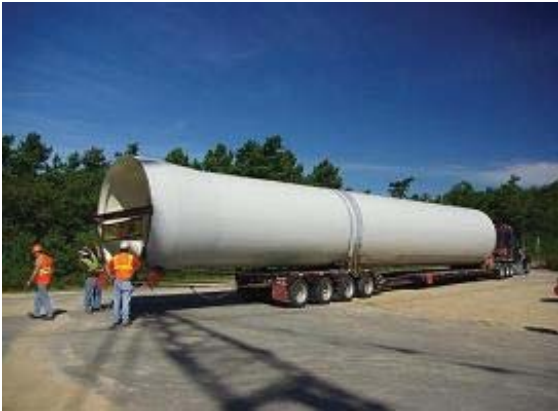
The 80-meter wind turbine tower began arriving at MMR in October 2009, in four sections. Transport involved securing state and local permits and tight scheduling to accommodate police escorts and inclement weather. Navigational challenges such as overhead utilities and bridges resulted in minor dents and scrapes to one section and temporary I-81 lane closure (due to damage of a New York bridge).
