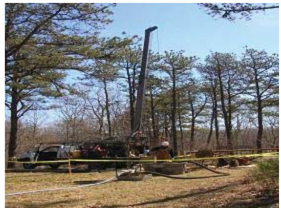
Use of biodiesel (B20) instead of conventional diesel to power the direct push rig and other equipment for well maintenance reduces onsite emission of air toxics and annually saves the project $2,000.
