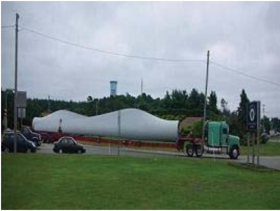
Three 123-foot epoxy/fiberglass blades were shipped to MMR from a manufacturing plant in Grand Forks, ND, in July 2009.
