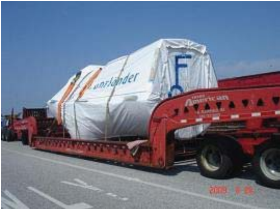
The 73-ton nacelle (generator) was shipped from Germany to MMR via the Baltimore Port in August 2009.
