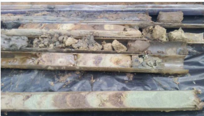
DNAPL: Borings from the pond area and process area contained creosote stringers.
