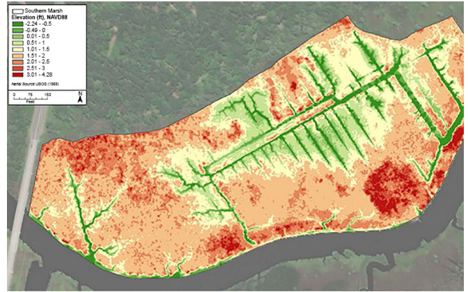
LiDAR-Based Topography Model: A digital elevation model representing bare earth at the southern marsh was generated from a 2014 LiDAR data set compiled by the National Oceanic and Atmospheric Administration (NOAA) and readily available in the NOAA DigitalCoast tool.
