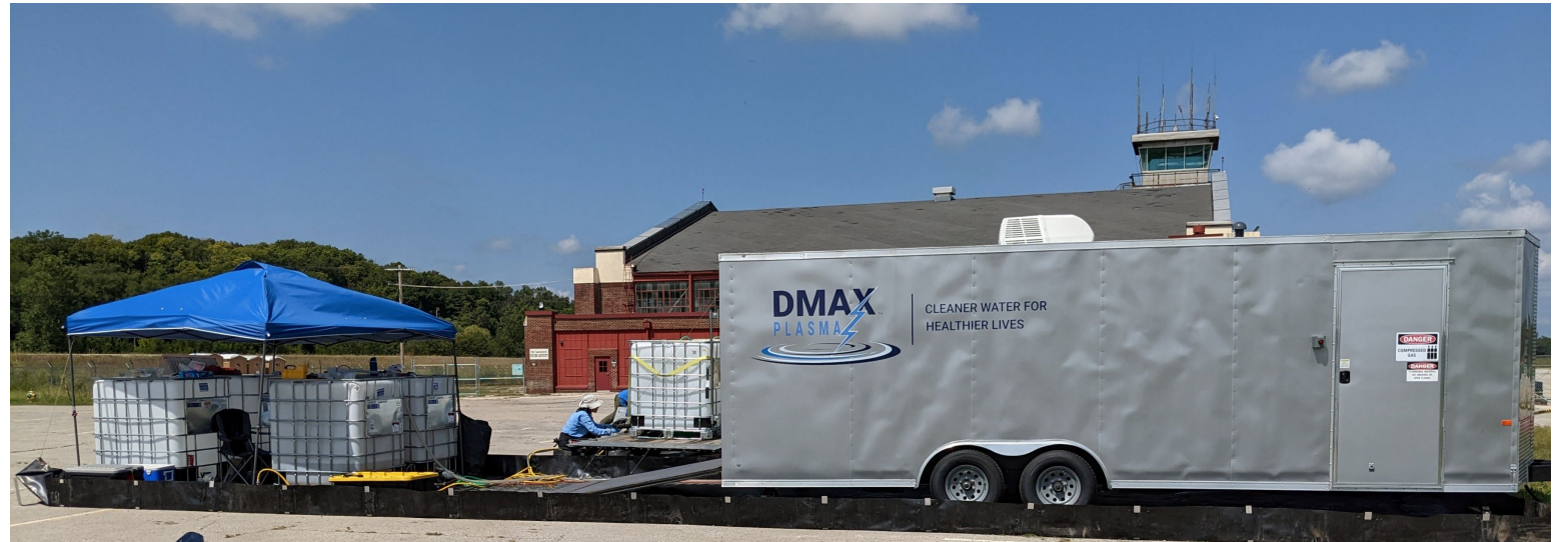
DMAX Plasma 4 th generation mobile treatment trailer
