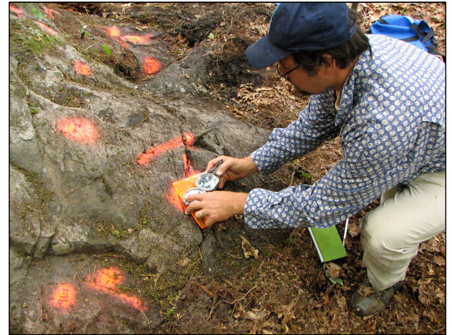
Measuring fractures with a Brunton (Bill Brandon, EPA)
