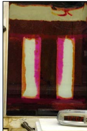
T = 6 hr w/ 2-hr EK (MnO 4 - flushing with EK )
