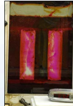
T = 12 hr w/ 8-hr EK (MnO 4 - flushing with EK )
