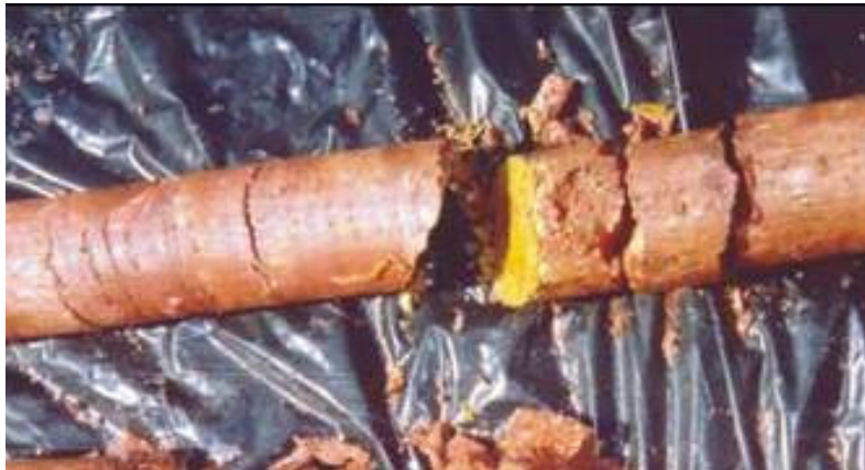
Figure 2. Weathered Bedrock at 20m bgs Presenting Fracture with Oxides
