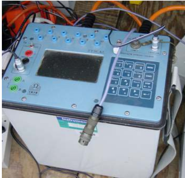
Figure 4. The IRIS Syscal Pro 10-channel resistivity instrument.
