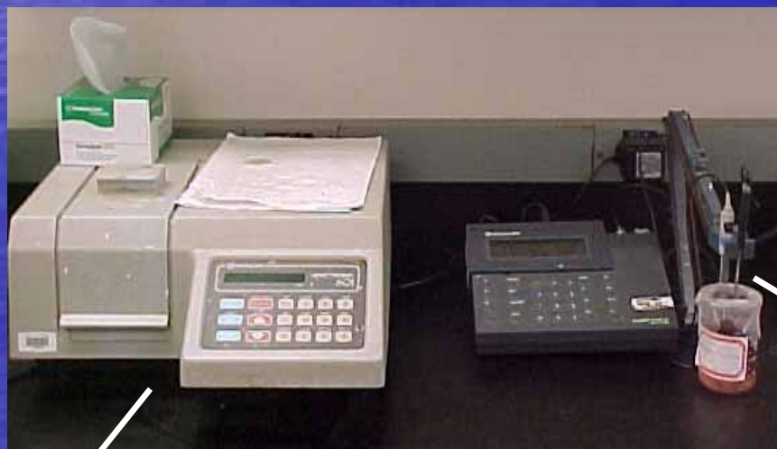
Spectrometer Used for H_2O_2 , KMnO_4 and Na_2S_2O_8 Analyses
