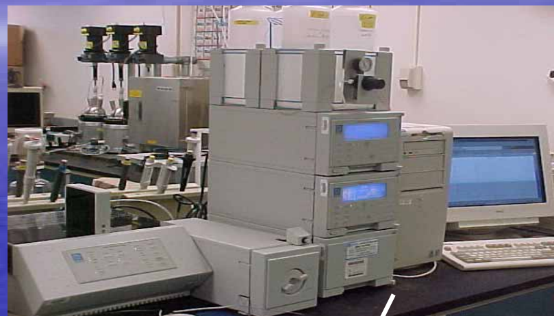
Ion Chromatography Used for Analysis of Chloride
