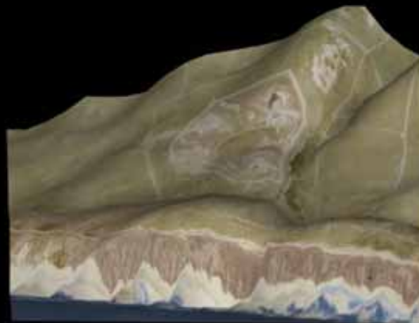
OVERLAYING A DIGITAL ELEVATION MODEL (with 5x vertical exaggeration)
