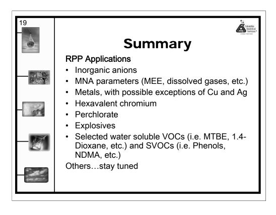
RPPS may be used to sample for most inorganics, but further studies are needed to determine suitability for some organics, especially less water soluble VOCs and SVOCs.
