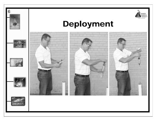
The RPPs are shipped in a water-filled pouch to ensure that air does not enter the pores. To deploy, cut open the outer bag with the red cap pointed up and the plug end down. Slip out of the bag which you can then discard. Attach the RPP to the deployment line using cable ties. It's very important to keep the red cap up and plug down. Gently lower the sampler down the well taking care not to jerk the line or hit the slides of the well to avoid weaping from the walls of the sampler.
