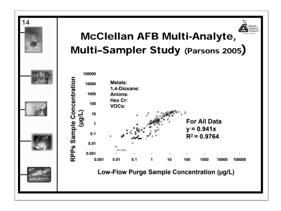
This study compared 4 passive sampling devices (PDB, Nylon-screen, regeneratedcellulose membrane sampler and the polysulfone-membrane sampler) and 2 equilbrated grab samplers (Hydrasleeve and Snap Sampler) against low-flow and conventional 3-volume well purging sampling. This graph depicts RPPs against lowflow sample results.
