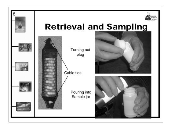
Use the same care when retrieving the samplers as deploying them. When the RPP appears at the top of the well, cut the cable ties holding the sampler to the deployment line, keeping the sampler in the same orientation. Cut away the cable ties that hold the mesh together at the top and the bottom of the sampler. Push down on the red cap, through the mesh, until the white plug is free of the mesh still keeping it in the same orientation (cap up, plug down).
