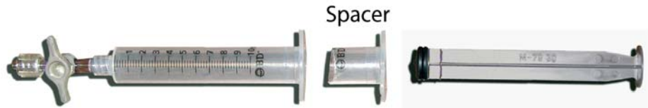
A. Exploded view of bag-less syringe H 2 sampler
