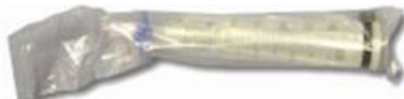
C. Deployed syringe in two LDPE sleeves
