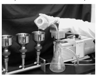
Step 3. Transfer filter to extraction tube containing glass beads, buffer and positive control DNA
