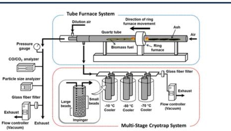
**Figure 1.** Diagram of the biomass combustion and smoke collection system. The tube furnace system consisted of a quartz tube and a ring furnace that traversed along the length of the quartz tube and was able to sustain stable flaming or smoldering phases consistently for 60 min. The multistage cryotrap system had three sequential impingers that were cooled cryogenically at –10, –50, and –70°C, permitting the capture of PM and semivolatile organic compounds from the biomass smoke emissions.
