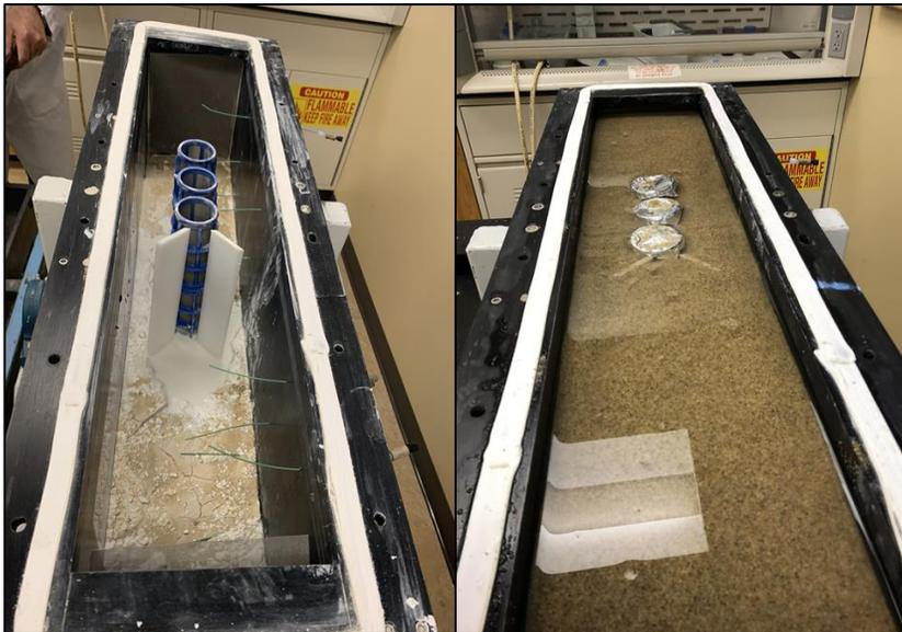
Top view of the PAM before packing with sand (left) and after (right)
