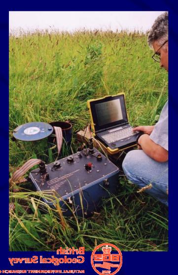
Electrode sensors have been permanently installed in landfill boreholes. Monthly monitoring helps to detect transient plumes and seasonal variations in leachate distribution within landfill
