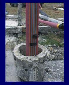
Electrodes on outside of PVC casing ensures electrical contact with surrounding material irrespective of water table
