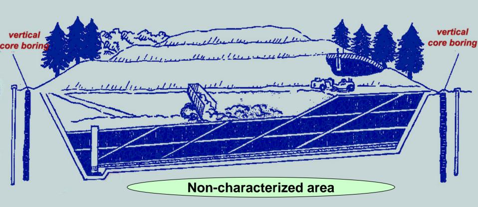
UMS can also recognize the underneath zone of the landfill achieving a more complete localization of the pollution leakage.
