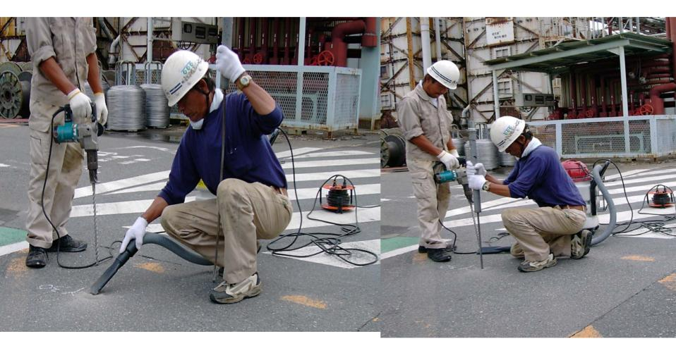
Measurement of GAS in a Factory under Operation (MOE : Demonstration Program for Low-cost and loading type soil monitoring and remediation technologies Provided by Suzuki (2003-2004)
