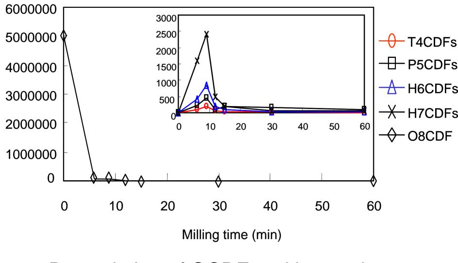
Degradation of OCDF and by-products during MC treatment of OCDF
