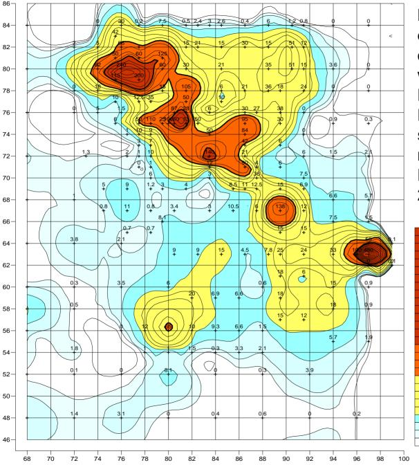
Horizontal distribution of TCE in soil gas determined by GAS without core boring (MOE : Demonstration Program for Low-cost and loading type soil monitoring and remediation technologies Provided by Suzuki (2003-2004)
