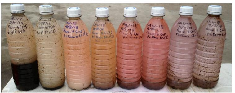
DNAPL recovery during ethanol push-pull test
