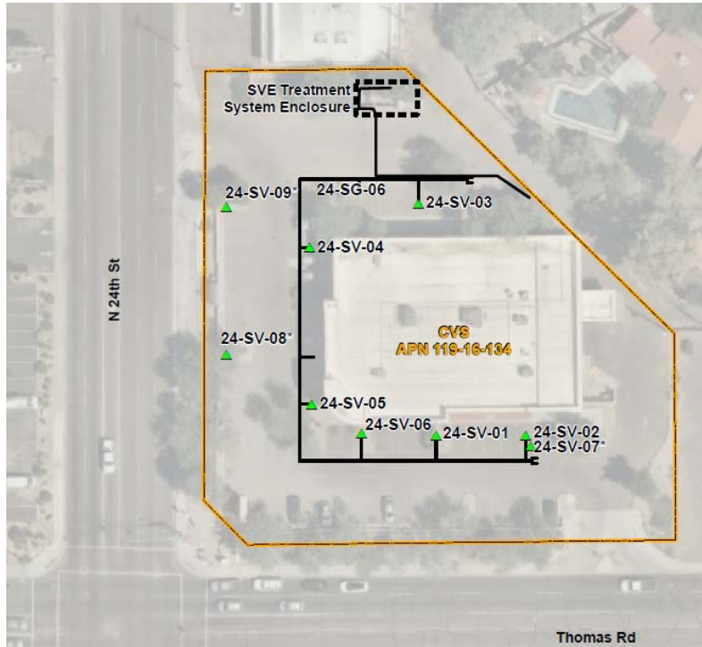
Former soil vapor extraction system
