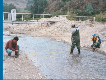
Manual stream gaging, Yanacocha, Peru
