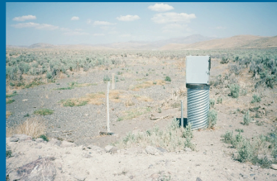
Gage for ephemeral stream near Betze Pit, Nevada
