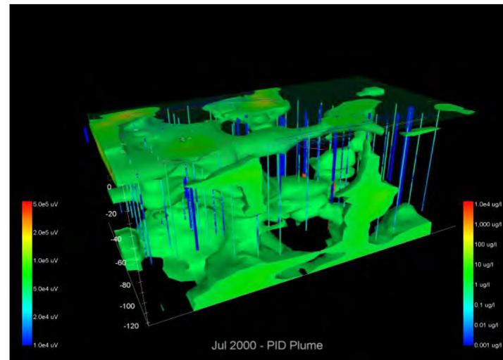
3-D plume visualization based on over 50 sampling locations
