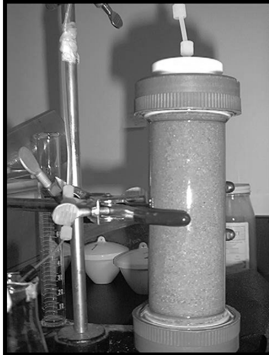
Figure 4-23. Photos of control setup. A) Overall setup. B) Sand column, ethanol influent, black substance at the entry to the sand, “generator” column. C) Sand column, groundwater only influent.
