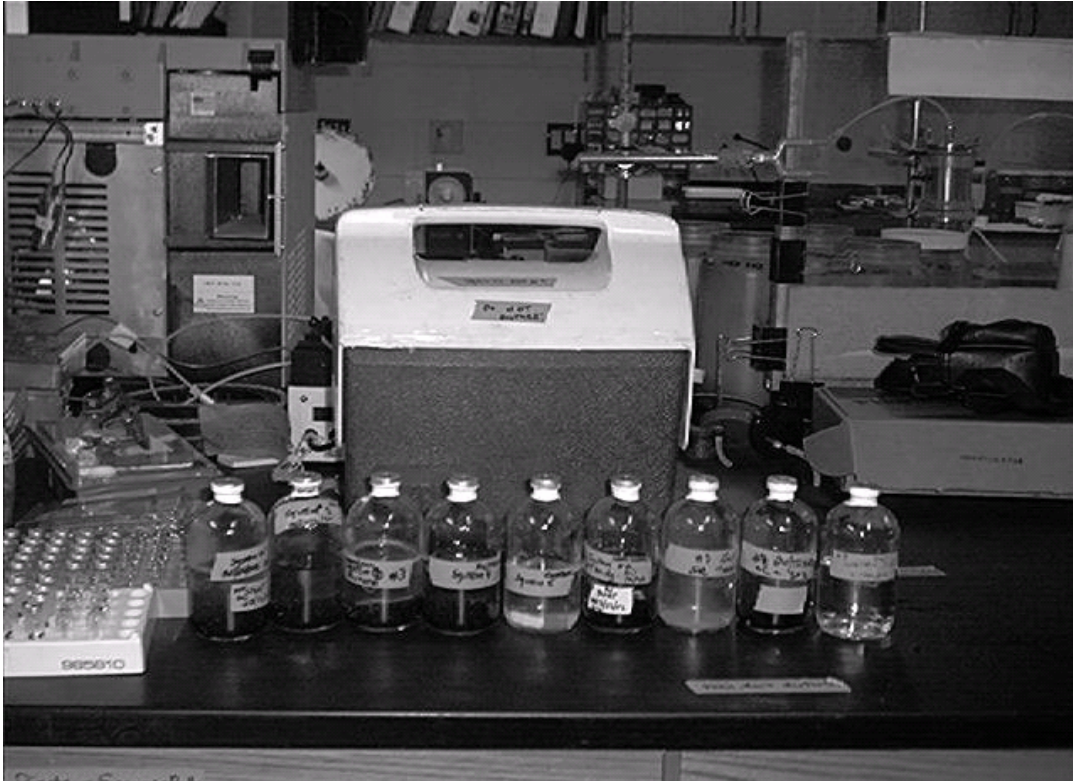
Figure 4-7. Series B oxygen-limited setup, 8 batch systems
