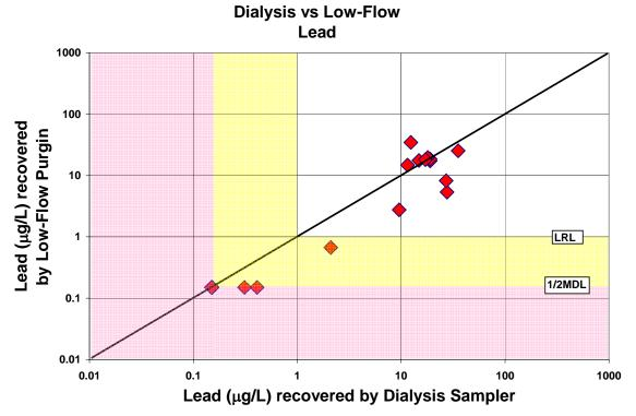
Figure A-70. Comparison of lead concentrations recovered by the dialysis sampler and low-flow purging
