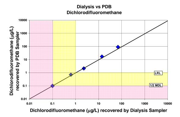
Figure A-15. Comparison of dichlorodifluoromethane concentrations recovered by the dialysis sampler and the polyethylene diffusion bag (PDB) sampler
