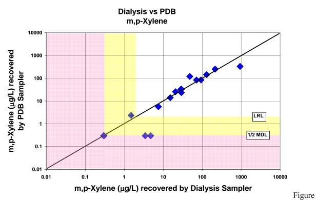
A-21. Comparison of m,p-xylene concentrations recovered by the dialysis sampler and the polyethylene diffusion bag (PDB) sampler
