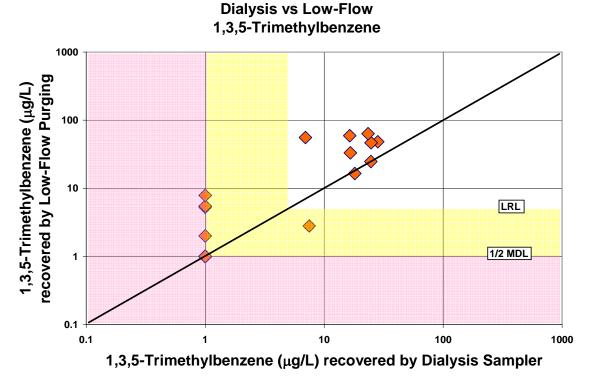
Figure A-8. Comparison of 1,3,5-trimethybenzene concentrations recovered by the dialysis sampler and low-flow purging
