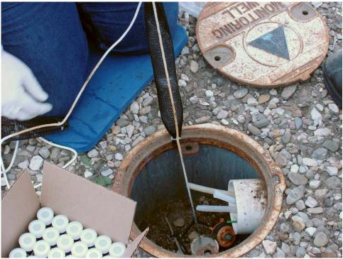
Figure 3-6. Removal Of Diffusion Sampler From A Well Prior To Sampling
