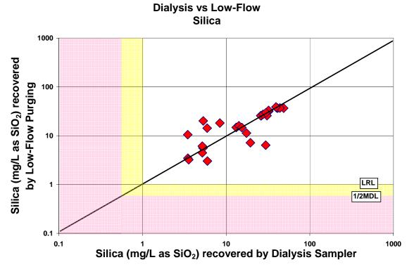
Figure A-60. Comparison of silica concentrations recovered by the dialysis sampler and low-flow purging
