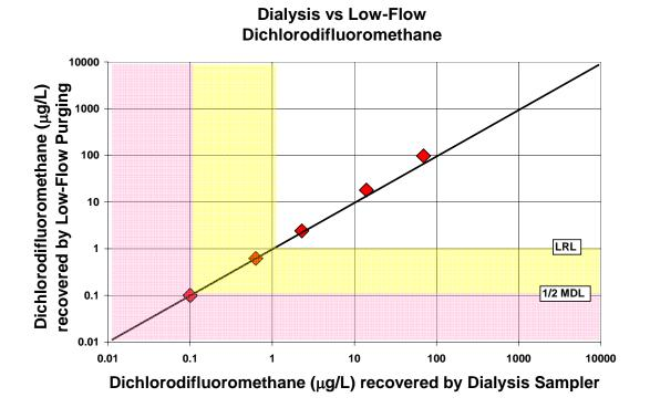
Figure A-16. Comparison of dichlorodifluoromethane concentrations recovered by the dialysis sampler and low-flow purging
