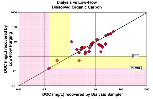
Figure A-78. Comparison of dissolved organic carbon (DOC) concentrations recovered by the dialysis sampler and low-flow purging
