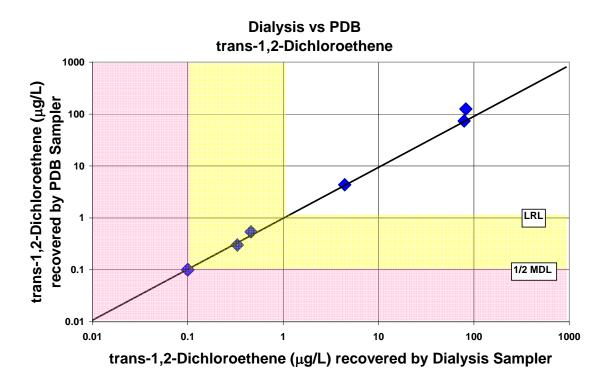
Figure A-45. Comparison of trans-1,2-dichloroethene concentrations recovered by the dialysis sampler and the polyethylene diffusion bag (PDB) sampler
