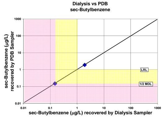
Figure A-35. Comparison of sec-butylbenzene concentrations recovered by the dialysis sampler and the polyethylene diffusion bag (PDB) sampler
