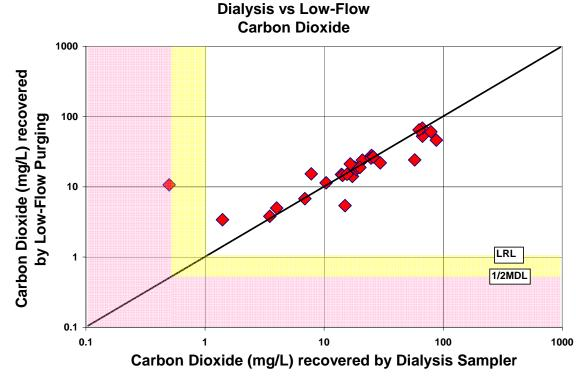
Figure A-74. Comparison of carbon dioxide concentrations recovered by the dialysis sampler and low-flow purging
