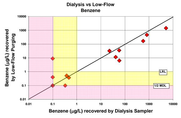
Figure A-10. Comparison of benzene concentrations recovered by the dialysis sampler and low-flow purging
