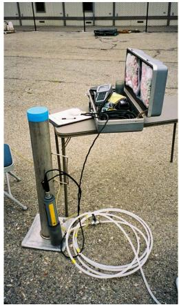
Figure 3-8. Flow Chamber And Multi-Parameter Instrument Used For Monitoring Field Parameters During Low-Flow Purging
