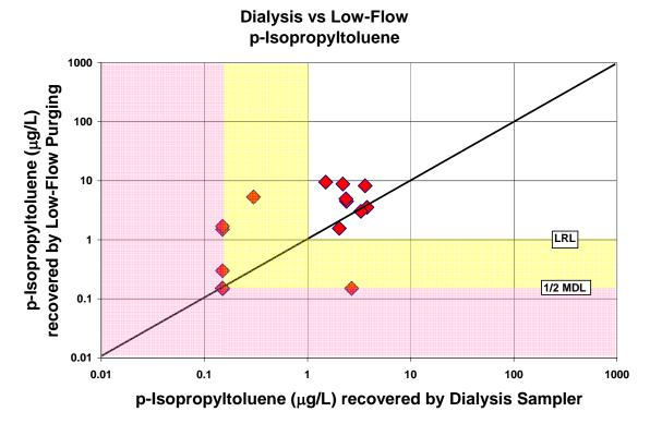
Figure A-34. Comparison of p-isopropyltoluene concentrations recovered by the dialysis sampler and low-flow purging
