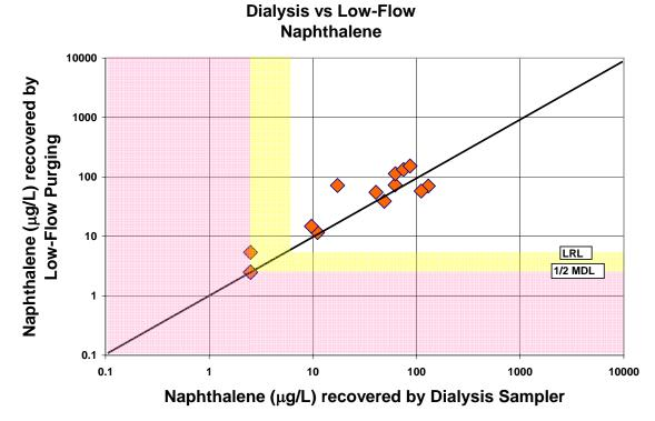
Figure A-26. Comparison of naphthalene concentrations recovered by the dialysis sampler and low-flow purging
