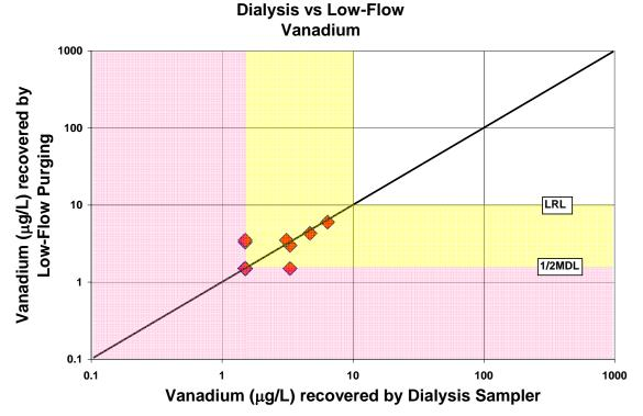
Figure A-72. Comparison of vanadium concentrations recovered by the dialysis sampler and low-flow purging
