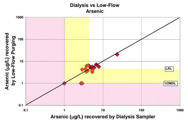
Figure 4-11. Dialysis Sampler Versus Low-Flow Purging Results For Arsenic
