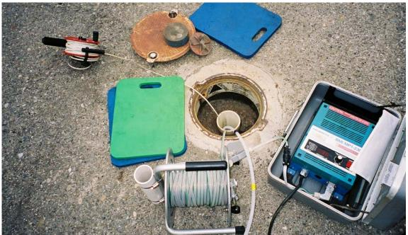
Figure 3-7. Low-Flow Purging Set Up For A 4-Inch Diameter Well. A Submersible Pump Is Being Used To Purge And An Electric Tape Is Being Used To Monitor Drawdown
