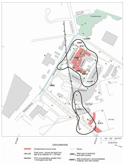
Figure 3-5. Wells Sampled As Part Of The Field Demonstration At Naval Air Warfare Center, West Trenton, New Jersey.
