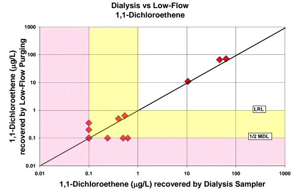
Figure A-4. Comparison of 1,1-dichloroethene concentrations recovered by the dialysis sampler and low-flow purging
