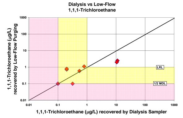
Figure A-2. Comparison of 1,1,1-trichloroethane concentrations recovered by the dialysis sampler and low-flow purging
