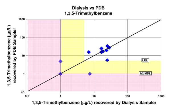
Figure A-7. Comparison of 1,3,5-trimethybenzene concentrations recovered by the dialysis sampler and the polyethylene diffusion bag (PDB) sampler
