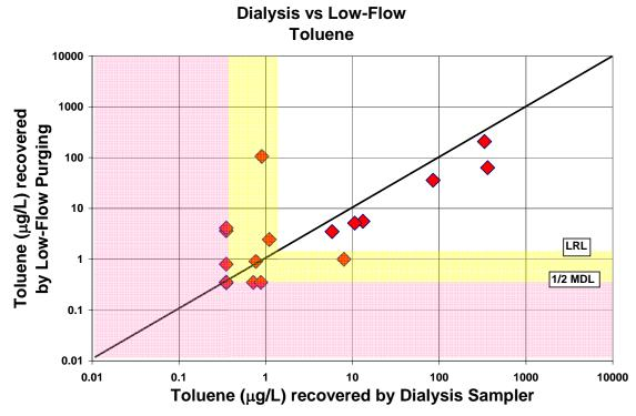
Figure A-44. Comparison of toluene concentrations recovered by the dialysis sampler and low-flow purging.
