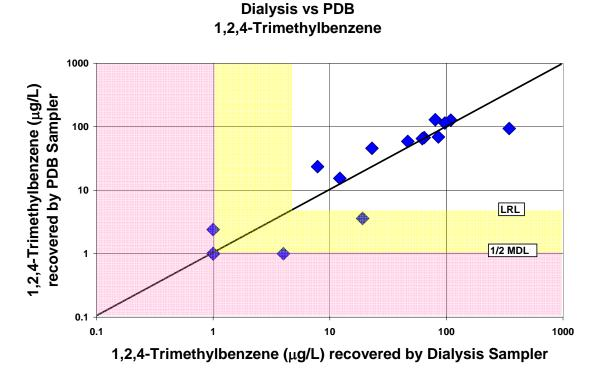
Figure A-5. Comparison of 1,2,4-trimethylbenzene concentrations recovered by the dialysis sampler and the polyethylene diffusion bag (PDB) sampler
