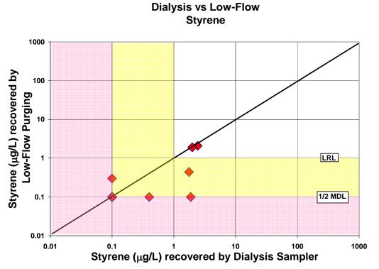
Figure A-38. Comparison of styrene concentrations recovered by the dialysis sampler and low-flow purging
