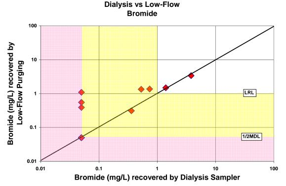
Figure A-58. Comparison of bromide concentrations recovered by the dialysis sampler and low-flow purging
