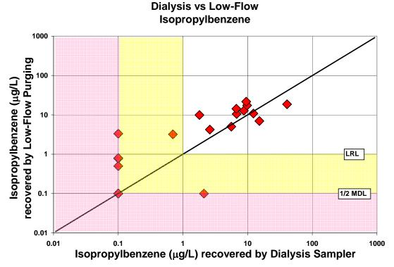
Figure A-20. Comparison of isopropylbenzene concentrations recovered by the dialysis sampler and low-flow purging
