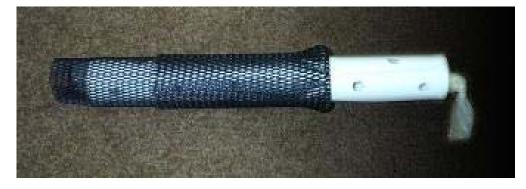
Figure 2-5. Regenerated Cellulose Dialysis Membrane Diffusion Sampler With Perforated PVC Pipe Support Inside the Membrane
