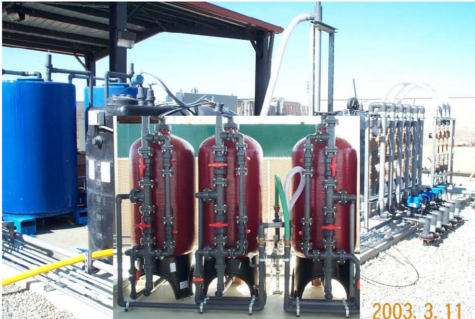
Figure 2-2. Small-scale ORNL Perchlorate Treatment Systems were Built and Demonstrated at Edwards Air Force Base (Gu et al., 2005)
