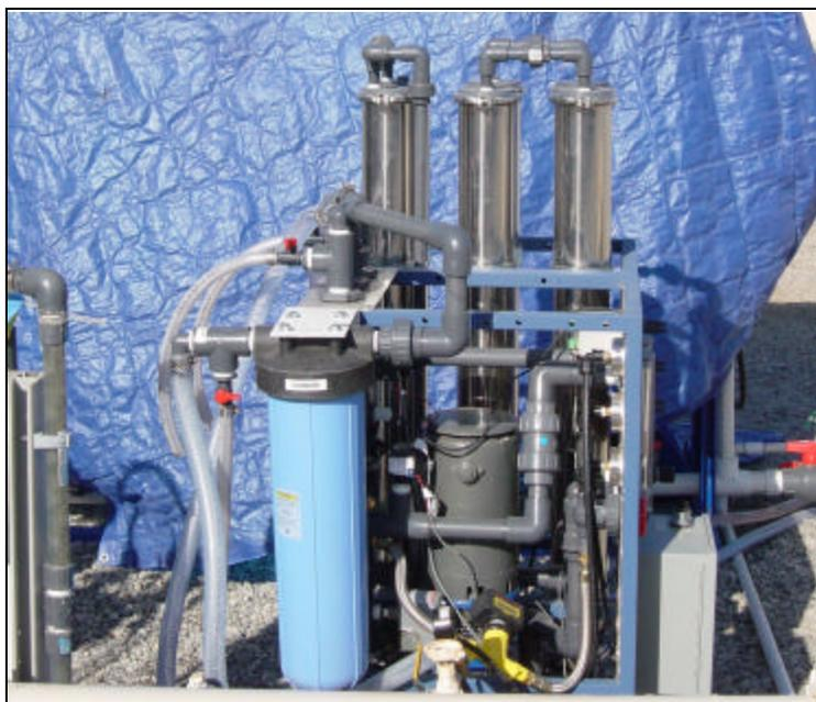
**Photograph 3: Pre-Filter to Watts Premier M-15,000 RO Treatment System**
