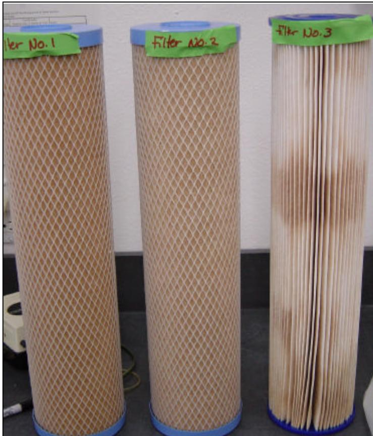
**Photograph 4: Watts Premier M-15,000 RO Treatment System Pre-filters**
