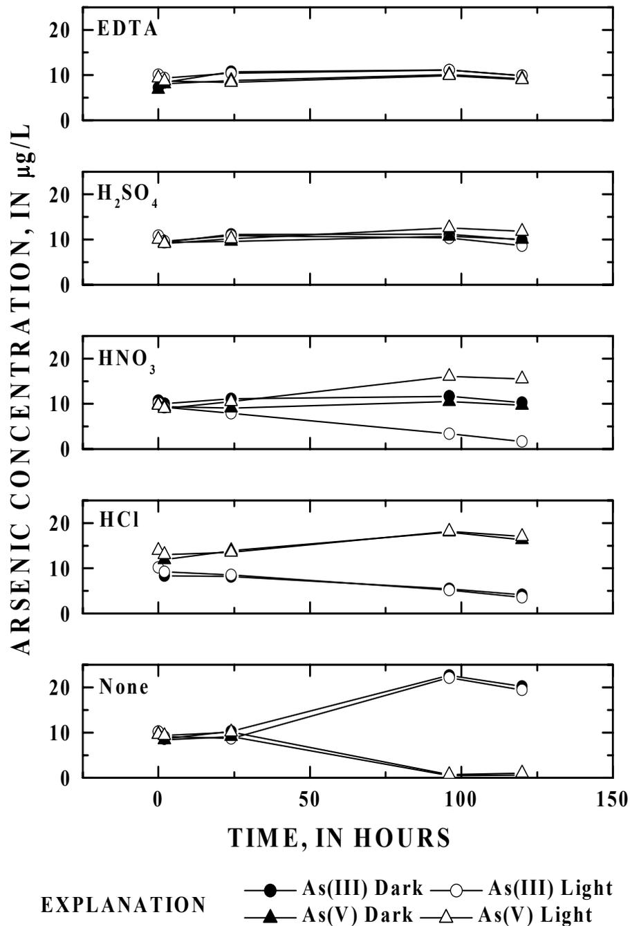
**Figure 8.** Ethylenediaminetetraacetic acid (EDTA), sulfuric acid (H<sub>2</sub>SO<sub>4</sub>), nitric acid (HNO<sub>3</sub>), and hydrochloric acid (HCl) as preservatives for arsenic speciation and the effects of ambient light. The experimental solution initially contained an equal distribution of As(III) and As(V) in reagent water. The top graph shows that EDTA preserved the arsenic distribution for 120 hours. Arsenic concentrations are in micrograms per liter (µg/L).
