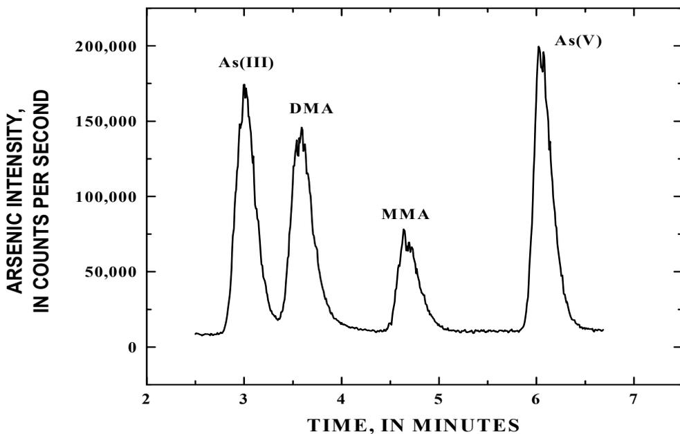
**Figure 1.** A typical chromatogram using the PRP-X100 column, a gradient phosphate mobile phase, and arsine introduction. The peaks represent a 100-microliter injection of a standard containing 10 microgram-arsenic per liter of arsenite [As(III)], dimethylarsinate (DMA), monomethylarsonate (MMA), and arsenate [As(V)].
