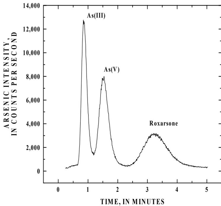
**Figure 3.** Typical chromatograms using the short LC-SAX column, an isocratic malonate/acetate mobile phase, and nebulizer introduction. The peaks represent a 100-microliter injection of a standard containing 10 micrograms-arsenic per liter of arsenite [As(III)], arsenate [As(V)], and roxarsone.
