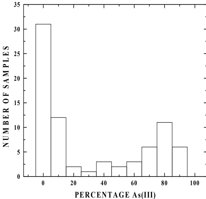
**Figure 10.** Distribution of As(III) percentage in ground-water and acid mine drainage samples.
