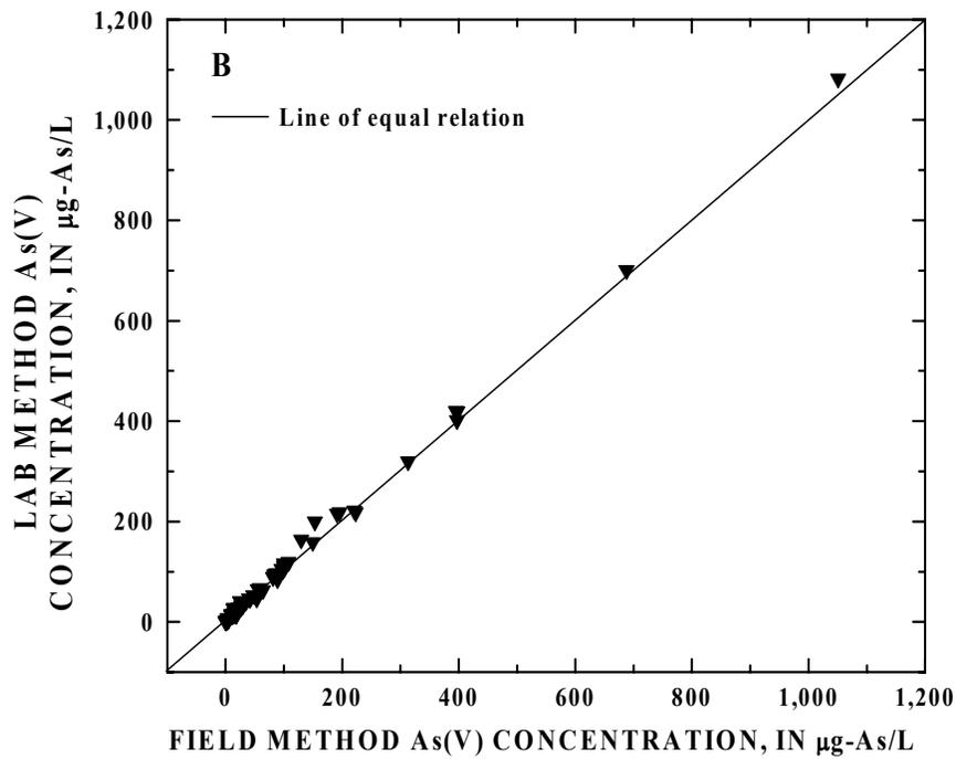
**Figure 11.** Linear regression analysis of laboratory and field dissolved As(III) [A] and dissolved As(V) [B] results for ground-water samples. Concentrations are in micrograms-arsenic per liter (µg-As/L).
