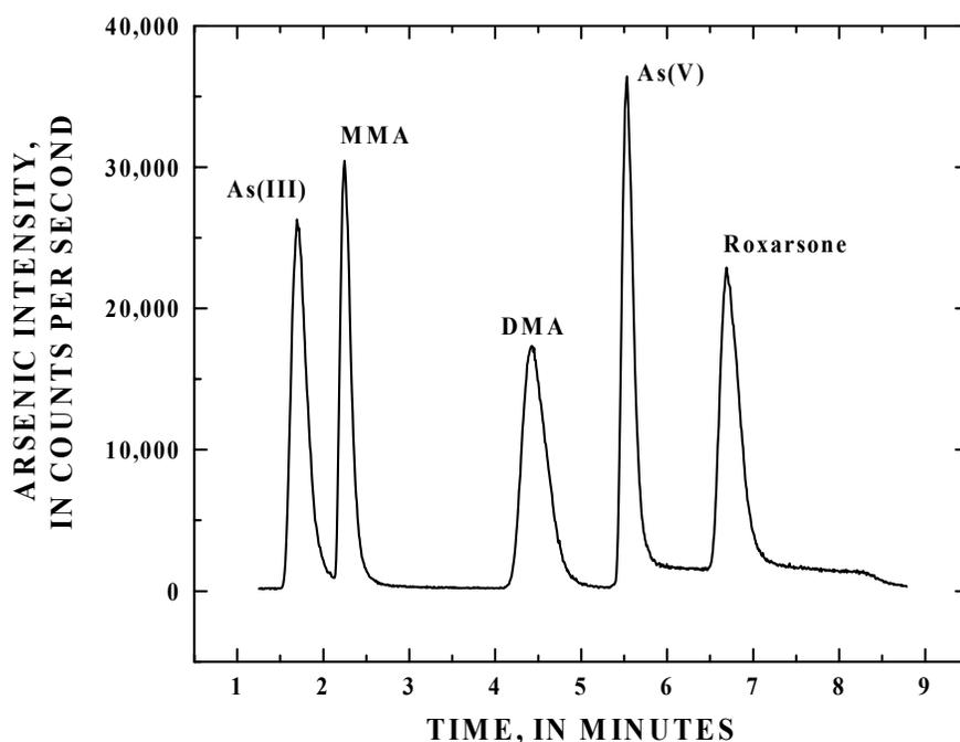
**Figure 2.** A typical chromatogram using the AS7 column, a gradient nitric acid mobile phase, and nebulizer introduction. The peaks represent a 100-microliter injection of a standard containing 10 micrograms-arsenic per liter of arsenite [As(III)], dimethylarsinate (DMA), monomethylarsonate (MMA), arsenate [As(V)], and roxarsone.
