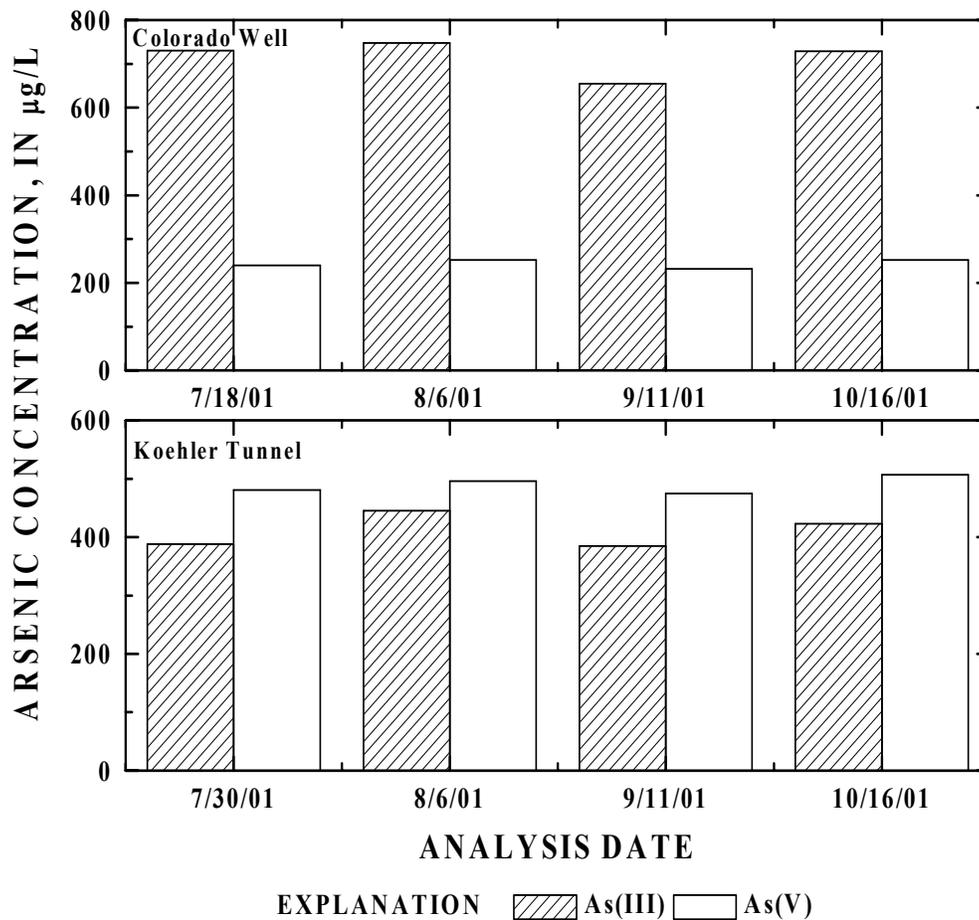
**Figure 14.** Preservation of arsenic species distribution for a 3-month period for a ground-water sample (Colorado Well) and an acid mine drainage sample (Koehler Tunnel). The Colorado Well and Koehler Tunnel samples were collected in opaque polyethylene bottles and preserved with EDTA on 7/18/01 and 7/27/01, respectively. Arsenic concentrations are in micrograms per liter ( $\mu\text{g/L}$ ).
