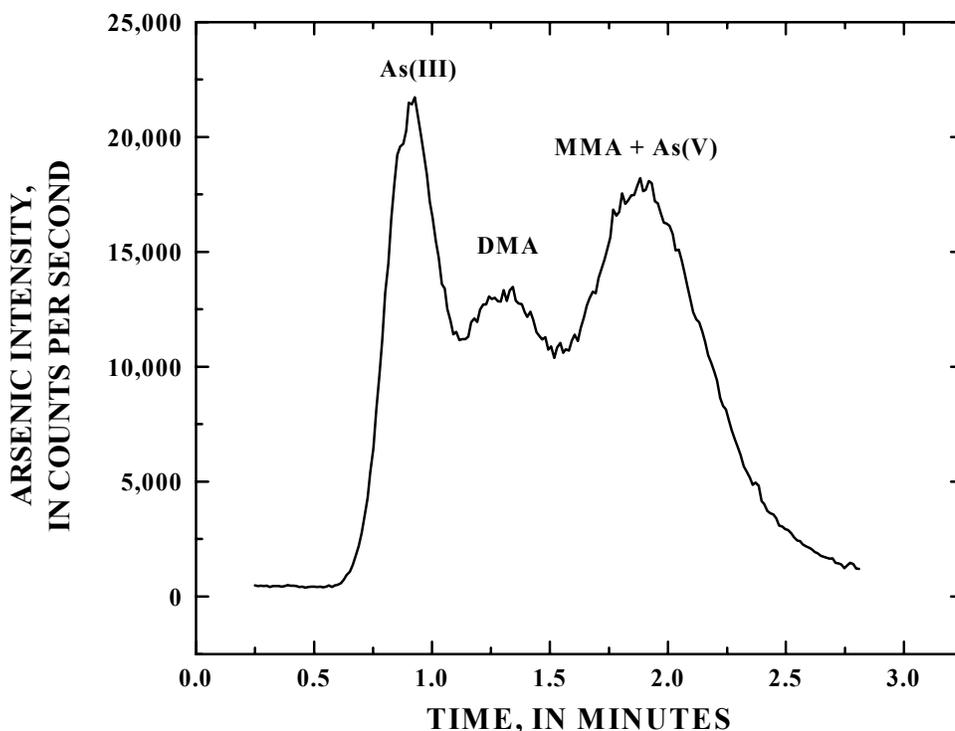
**Figure 4.** Methylated arsenic species are not resolved from the inorganic arsenic species when using the short-column laboratory method (I-2192-02). Dimethylarsinate (DMA) is not resolved from arsenite [As(III)] and monomethylarsonate (MMA); MMA is not resolved from arsenate [As(V)].
