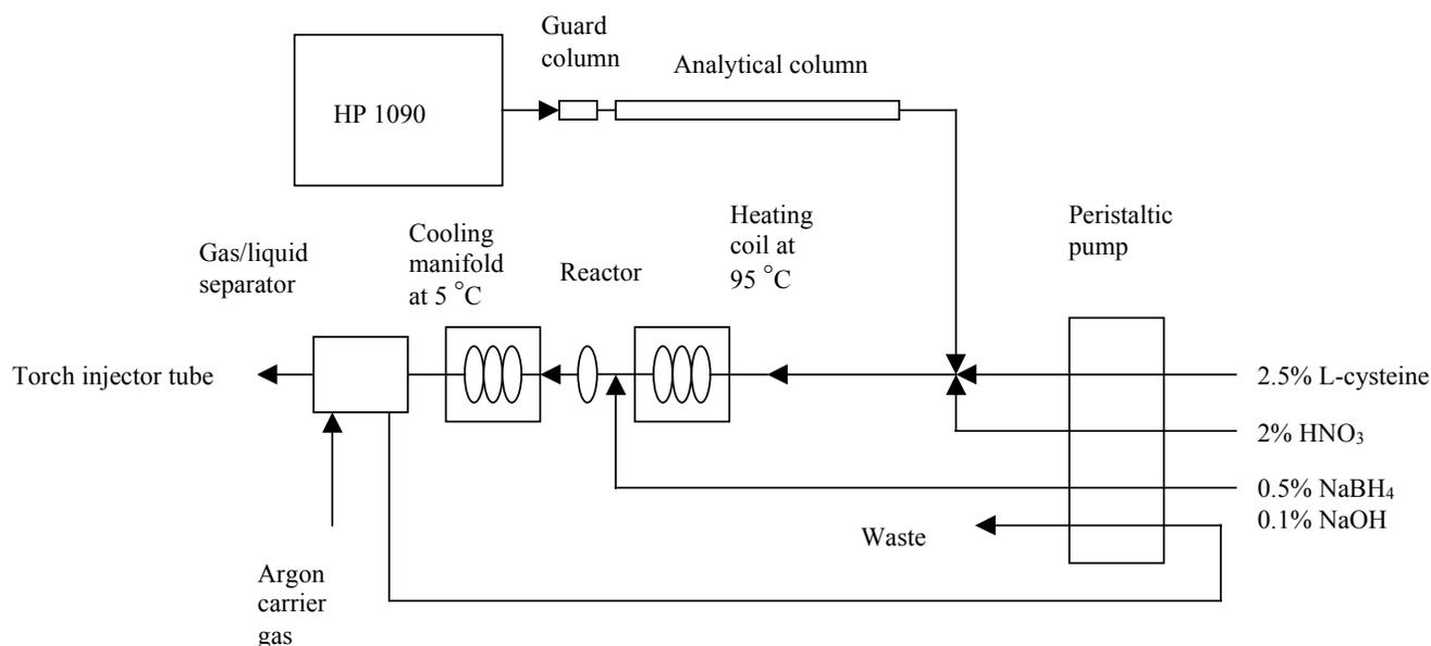
**Figure 6.** Ion chromatography, arsine generation, and inductively coupled plasma–mass spectrometric system. Reagent concentrations are given in weight percent (%) and temperature is in degree Celsius (°C).
