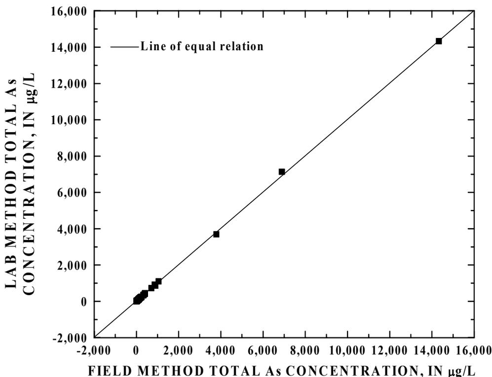
**Figure 13.** Linear regression analysis of laboratory and field total dissolved arsenic [As(III) plus As(V)] results for all test samples. Arsenic concentrations are in micrograms per liter ( $\mu\text{g/L}$ ).
