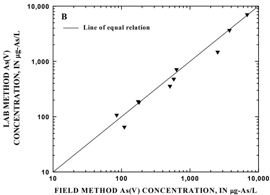
**Figure 12.** Linear regression analysis of laboratory and field dissolved As(III) [A] and dissolved As(V) [B] results for acid mine drainage samples. Concentrations are in micrograms-arsenic per liter (µg-As/L).
