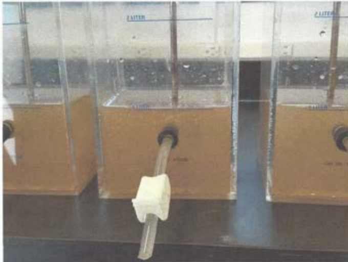
Test Jars showing leachate dosed with lime and ferric chloride:
