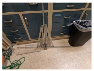
Figure ES-2. The Modified Multisampler Anchor without PE Sheets in the Laboratory.
