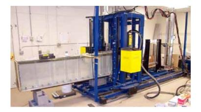
Figure 36 - Intermediate scale tank mounted on the x-ray platform.
