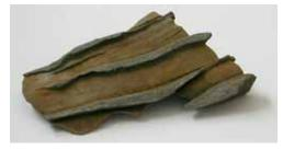
Figure 19 - Interbedded sandstone and shale, shown as an example of Type III media. SOURCE: Reprinted, with permission, from http://geology.about.com. © 2004 About.com.
