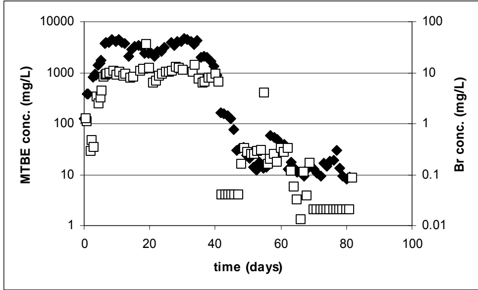
Figure A-6c. MTBE (black diamonds) and bromide (open squares) concentrations in the effluent of Tank 6a. MTBE contaminated water (including bromide) was fed from day 1 to day 25, after which water with neither contaminant nor bromide was fed to this tank until the end of the experiment.
