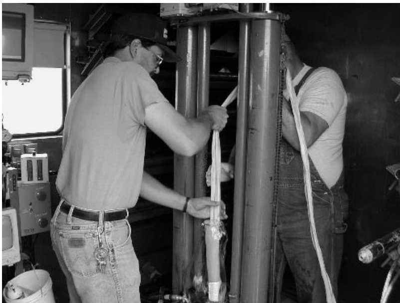
Figure 5. The membrane is retrieved by inversion.
