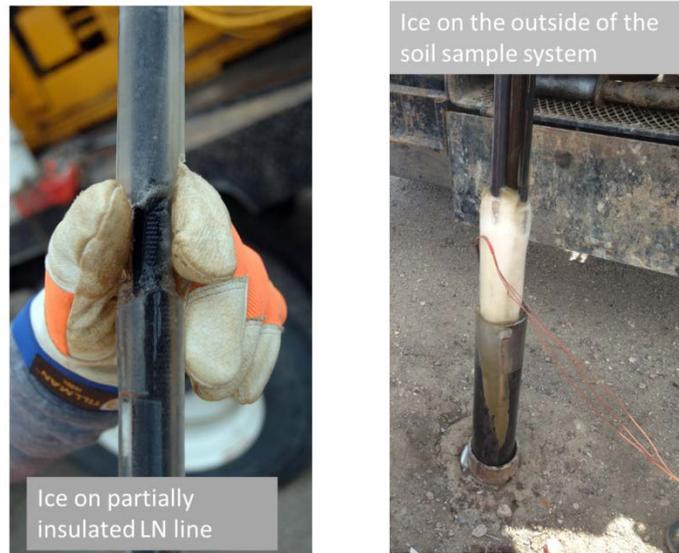
**Figure 3-16. Downhole ice locking**
