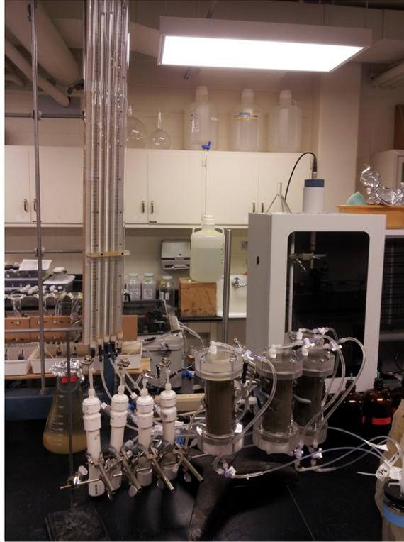
Figure 4-9. Falling head test station
