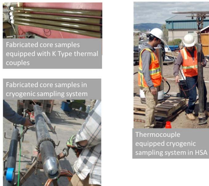
**Figure 3-13. Fabricated core samples**
