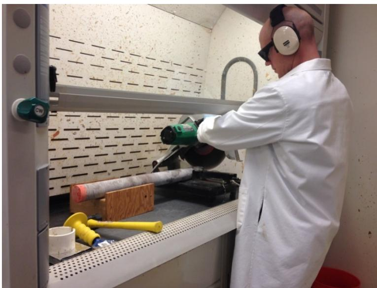
Figure 4-3. Photograph of frozen-core cutting
