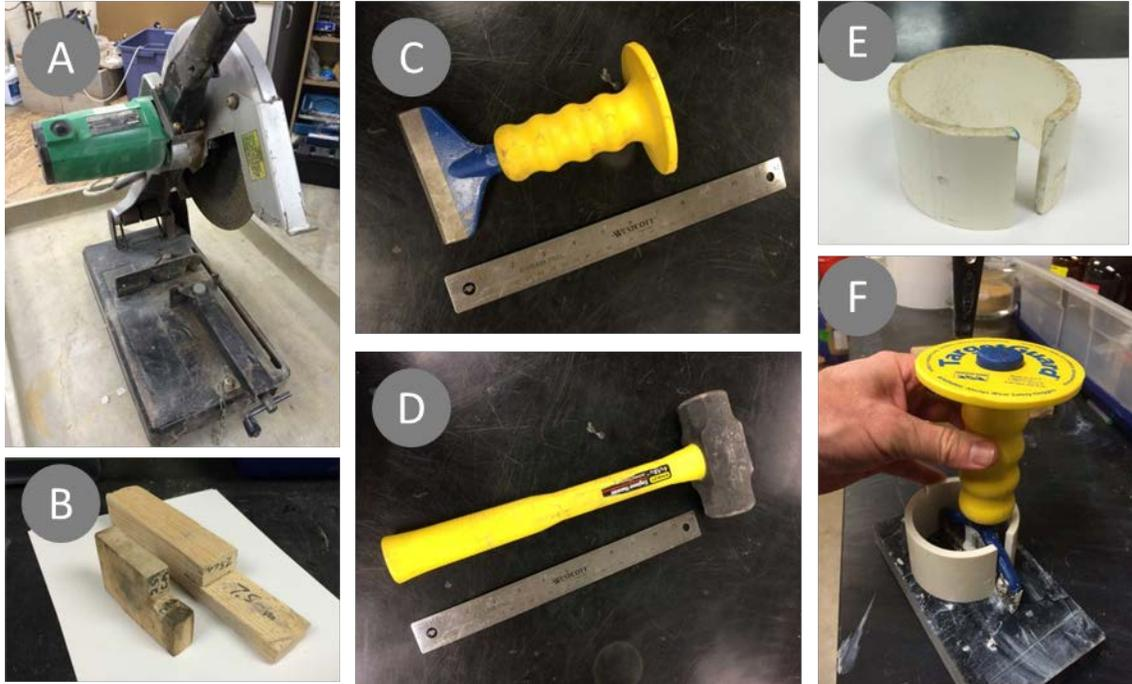
**Figure 4-1. Materials and equipment used for high-throughput core processing. The following are shown: (A) cut-off saw, (B) stop blocks, (C) chisel, (D) hammer, (E) PVC pipe, cut to size, and (F) entire apparatus used for sub-dividing frozen core discs.**
