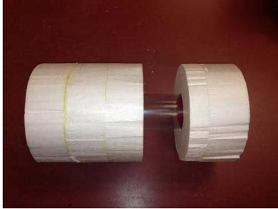
Figure 5-1. Styrofoam insulation for keeping the core frozen during MRI
