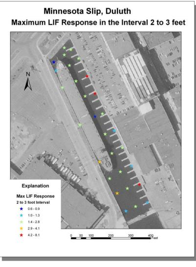
Figure 14: Maximum LIF Response Detected in Second and Third foot of Sediment.
