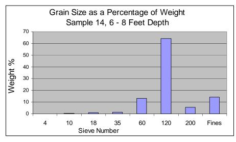
Figure 18: Gain Size Weight Distribution for Sample 14, 6 – 8 feet.
