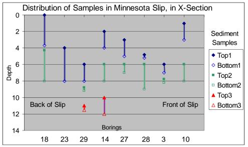
Figure 17: Distribution of Sediment Samples, by Depth and Location in the Slip.
