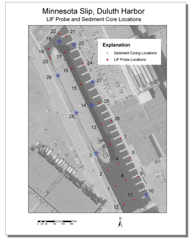
Figure 7: Location of LIF Probes and Sediment Cores.
