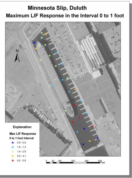
Figure 13: Maximum LIF Response Detected in Top Foot of Sediment
