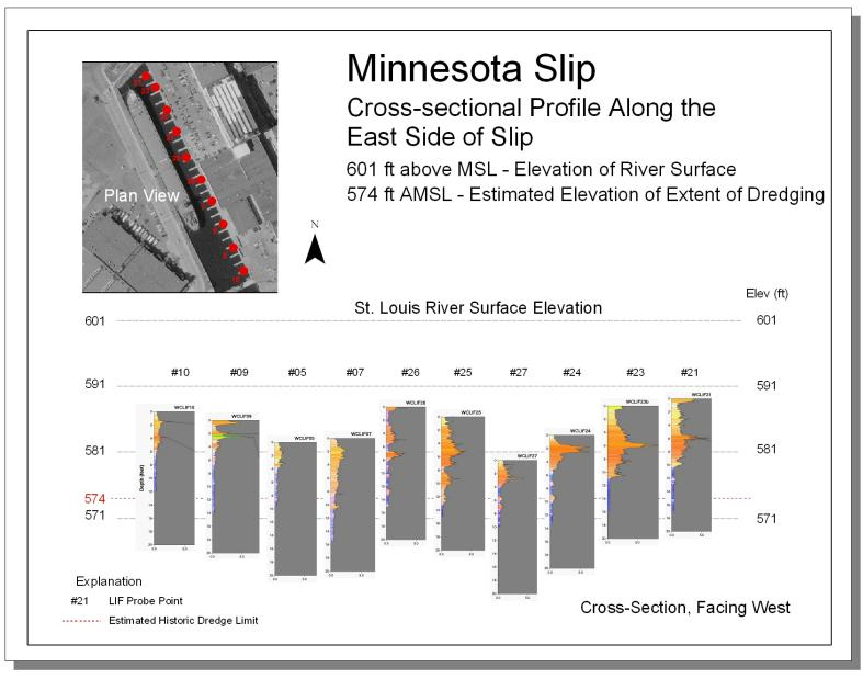
Figure 12: Cross-section Along the Eastern Wall of the Slip, Featuring LIF Response Records.
