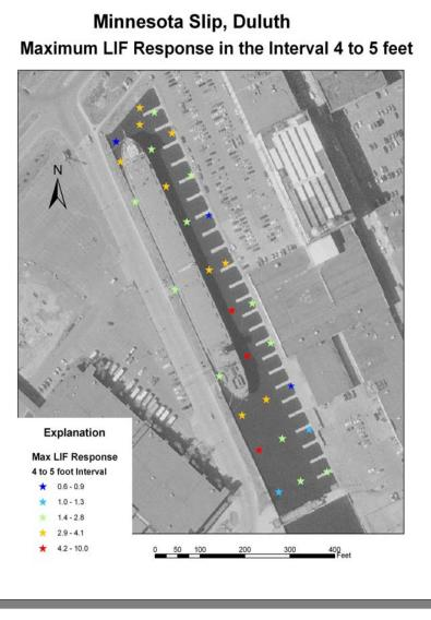
Figure 15: Maximum LIF Response Detected in Fourth and Fifth foot of Sediment.
