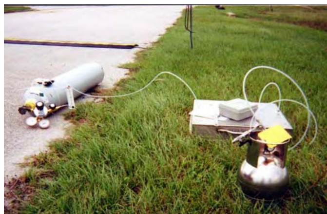
Figure 4-7. Surface Emissions Testing at Launch Complex 34
