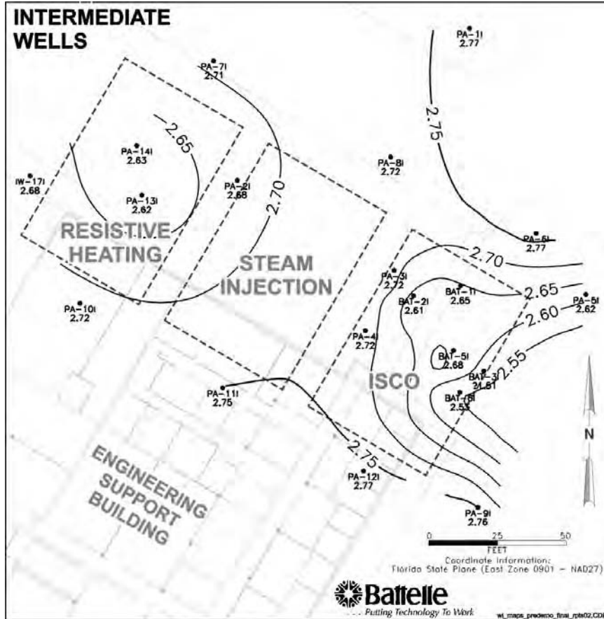
Figure 2-8. Pre-Demonstration Water Levels (as Elevations msl) in Intermediate Wells at Launch Complex 34 (September 1999)
