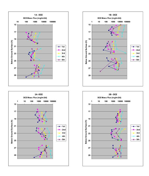
Figure 5-15. PFM DCE Flux Profiles for 5 Deployment Periods.
