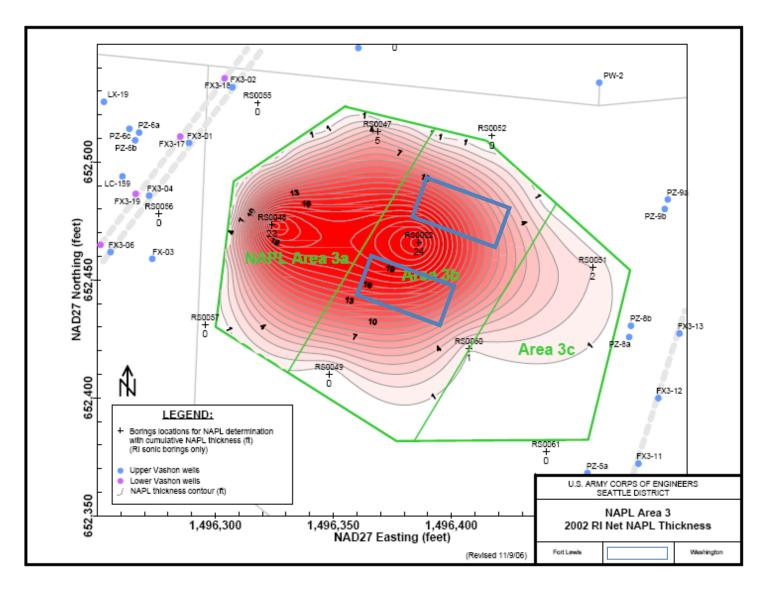
Figure 4-3. Inference of NAPL Distribution Within NAPL Area 3 Based on Data Gathered During the Phase 2 RI (2002) (USACE, 2008). Boxes Highlighted in Blue Indicate Target Treatment Cell Locations.
