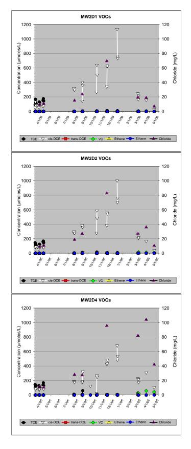
Figure 5-13. Molar Mass Plots of TCE and Reductive Daughter Products During Phases 2 and 3 of the Demonstration at MWD in Treatment Cell 2.
