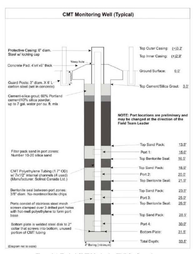
Figure 2-1. Typical CMT Monitoring Well Configuration.
