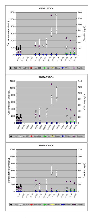
Figure 5-12. Molar Mass Plots of TCE and Reductive Daughter Products During Phases 2 and 3 of the Demonstration at MWA in Treatment Cell 2.
