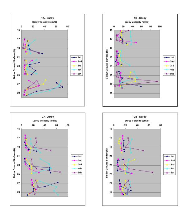
Figure 5-16. PFM Darcy Velocity Profiles for 5 Deployment Periods.
