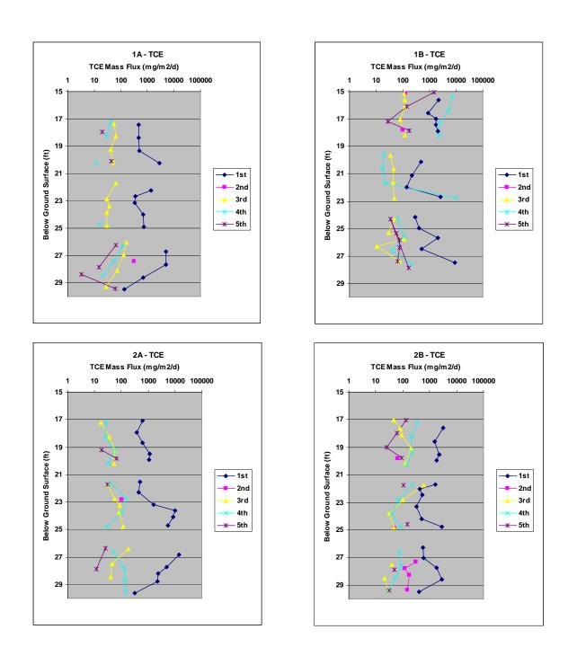
Figure 5-14. PFM TCE Flux Profiles for 5 Deployment Periods.
