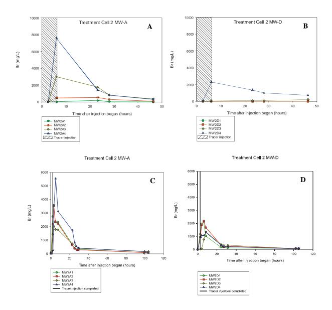
Figure 5-5. Comparison of Vertical Distribution of Tracer in Monitoring Wells A and D in Treatment Cell 2 Following Bromide Injections in the Original (A and B) and New (C and D) Injection Wells.
