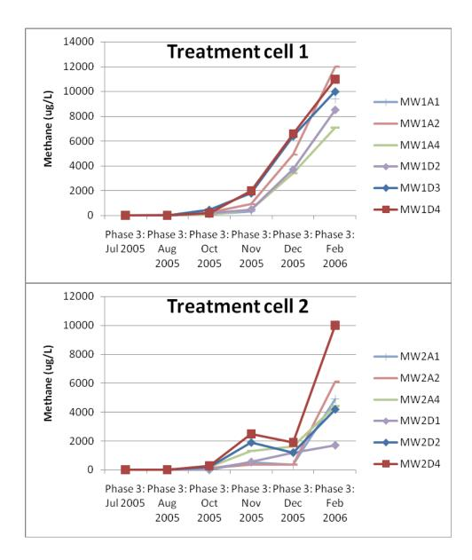
Figure 5-8. Methane Production Observed at Discrete Vertical Depths During Phase 3.
