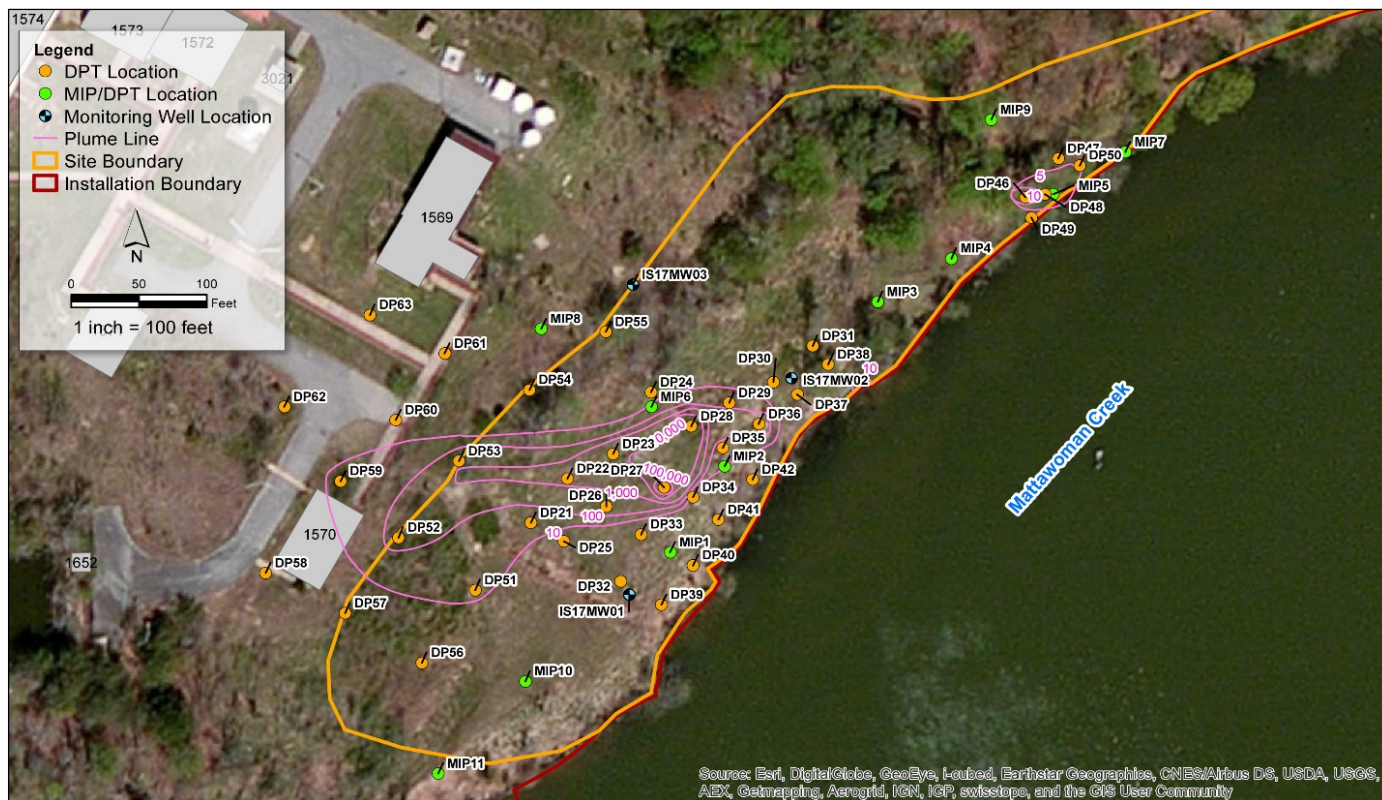
Figure IH-3a. Indian Head Site 17 TCE Plume, Upper Surficial Aquifer (2005)
