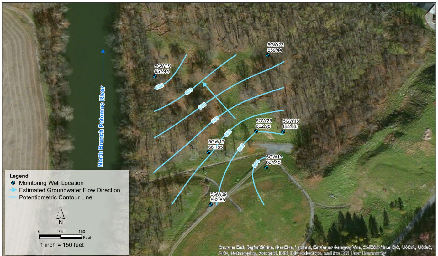
Figure AB-2. ABL Site 5 Groundwater Contour Map (2012)
