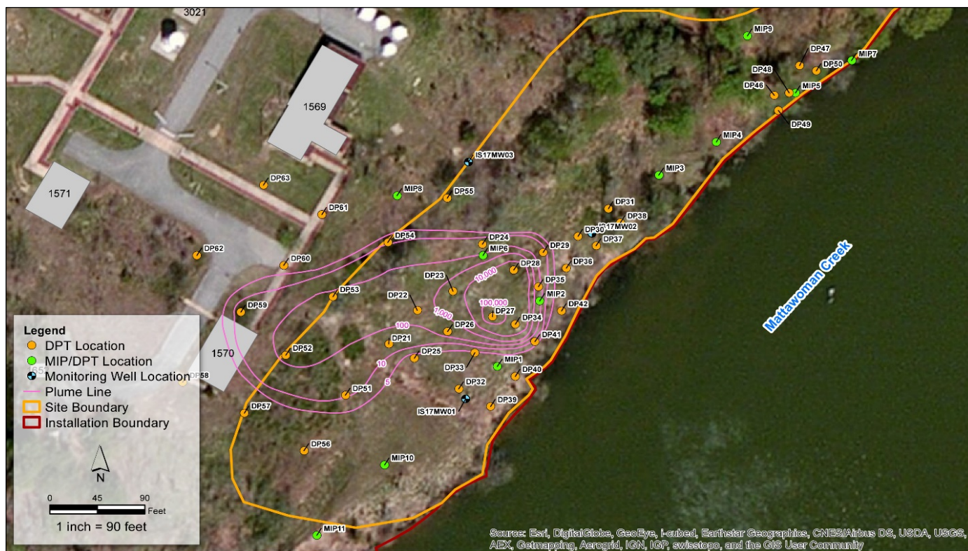
Figure IH-3b. Indian Head Site 17 TCE Plume, Lower Surficial Aquifer (2005)
